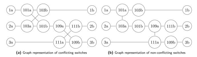
Figure 2-2: Modelling the switches in a shunting yard in a graph
