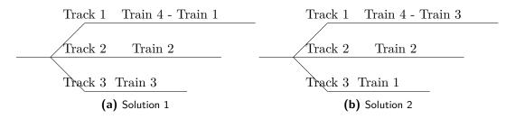
Figure 1-3: Example shunting yard topology
